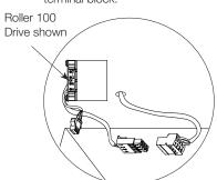
Note: Arrange wires in a location that prevents them from interfering with moving shade or drape.
